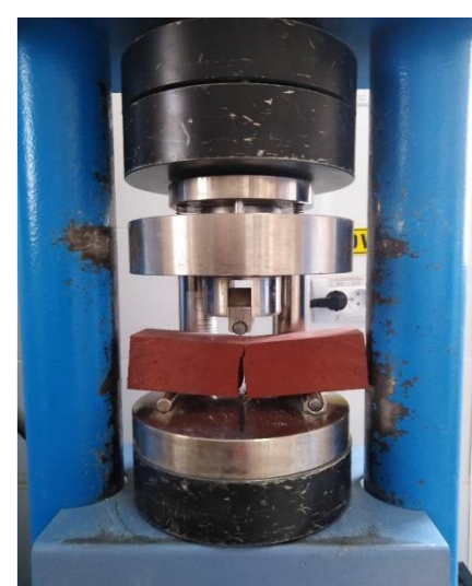
Figure 8. Testing machine for measure flexural strength.
