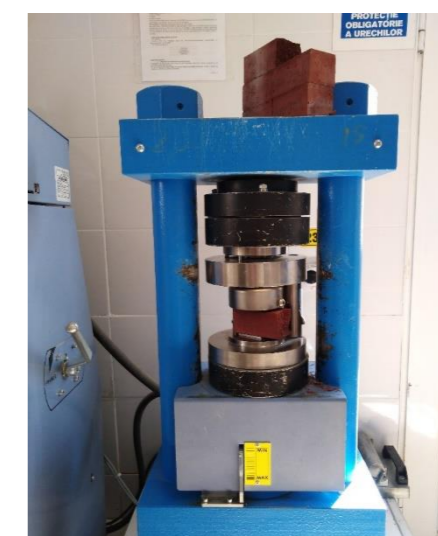
Figure 7. Testing machine for measure compressive strength.
