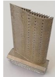
Hardware developed by LPBF in Inconel 625. Credit: COMOTI
