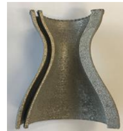
Hardware developed by LPBF in Inconel 625. Credit: COMOTI
