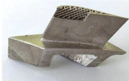
Hardware developed by LPBF in Inconel 625. Credit: COMOTI
